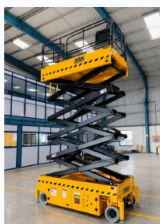
Self-Propelled Scissor Lifts 300 kg · Lift up to 14000mm
